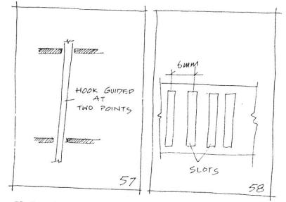
Slots, long enough to facilitate the pivoting of the hooks on the shaft and wide enough to just let the hooks move freely in them were punched out from a MS sheet using a die punch. 2 such sheets were enough to guide the hooks.[58]
