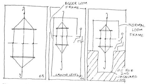
There would be a space problem because of the harness. Even if the length of the harness is reduced because of the new 'fatti board' solution, the total space required by two such harnesses, that of the top and bottom mechanisms, would be considerable.
