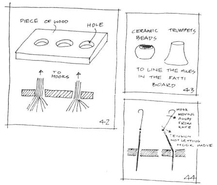
One problem which was raising its head constantly was that the effort required for moving the hooks off the knife (i.e. the effort required for rotating the selection device which would be rubbing against the hooks) was becoming considerable.
