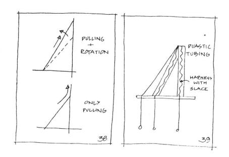
The cause of the height problem was identified as the geometry of the harness that was being pulled up as well as being rotated.[38]
