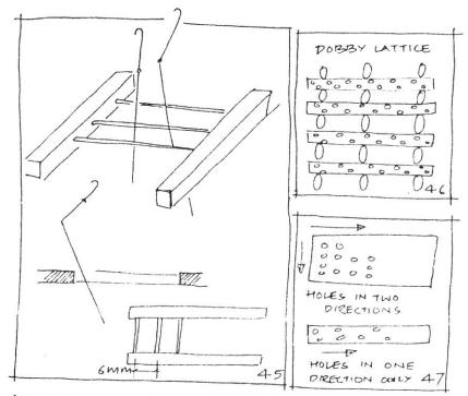
has holes spaced out by 6 mm centre to centre.
