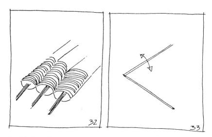
In Tistou the transverse threads were being laid across the needles and were getting crimped by them.
