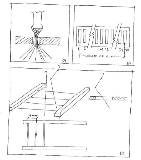
be able to punch out 80 holes in a length as much as that of a slat instead of holes at every 6 mm. [61]
