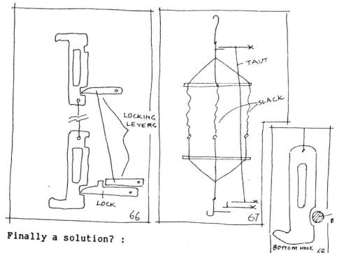
One locking system thought up along the way was based on a different principle.
