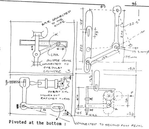
In this machine the dobby cylinder moves in an arc with the pivoted end at the bottom.
