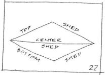
Because the threads in the normal bottom shed are distorted out of shape, the tension in them tries to pull them up. It is very important for them to remain in a clean bottom shed line is required. If the threads are not at the same level, the shuttle flying over them will get caught in them and break them.[23 & 24]
