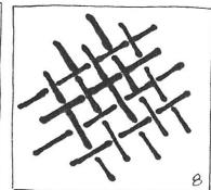
Warp passes through the eyes in the heald wires, alternating between the two frames.[9]
