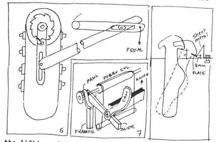
the lifting of knives and the above rotation of dobby cylinder can be synchronised then it could be tried out.
